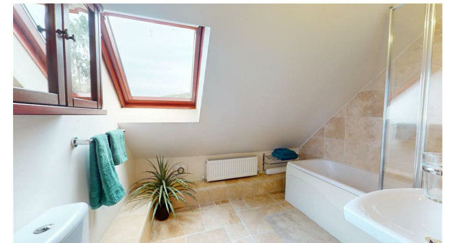
White suite comprising panelled bath with bi fold screen and combination shower and tap unit, pedestal wash basin and WC, Velux roof light, extractor fan, panelled radiator.
